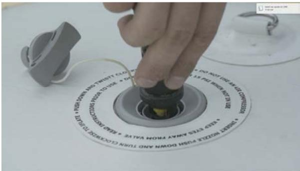
5. Stand the pump on hard, level ground and start to pump. The first time you inflate the Floating Deck will require more effort than subsequent inflations.
